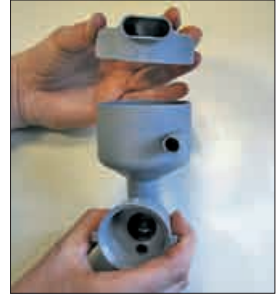
2-piece mixer jug All openings facing into same direction..
