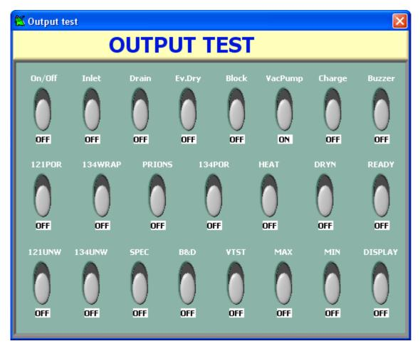
ON/OFF turns on the remote control switch (see page 24 of the STERILCLAVE SERVICE MANUAL). INLET turns on the sterilizer's A loads: the inlet solenoid valve EV1 and the water inlet pump (see page 24 of the STERILCLAVE SERVICE MANUAL).
