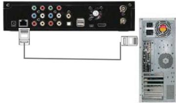
Connect LAN cable to the LAN ports between PBR-500 and PC.
