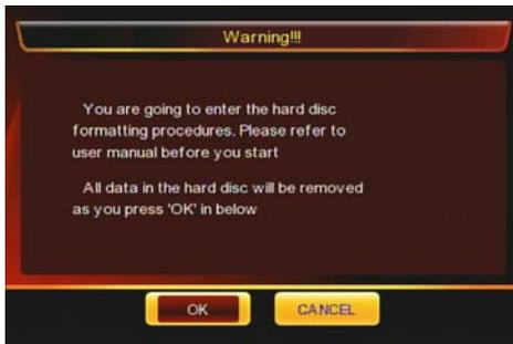
① Press [OK] to start a HDD format.
