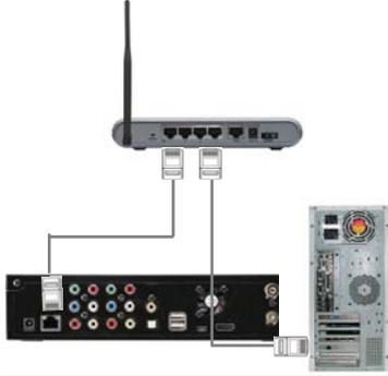
Connect LAN cable to the LAN ports between a Router or Hub and PBR-500.
