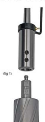
TAP50 uses the 5 Morse Taper spindle drilling. To be used with metal cutters, there is a necessity to use a 1.1/4" adapter. For this application a 1-1/4" Weldon Shank is the most common. This shank has the dimension of Ø31mm, 75 x 60mm and has 2 surfaces for the locking screws.
