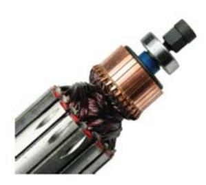
With regular use, the armature should be checked at least once per month. Look for visible damage or wear to the armature body and the commutator (commutator are brass plates which the brushes are touching).
