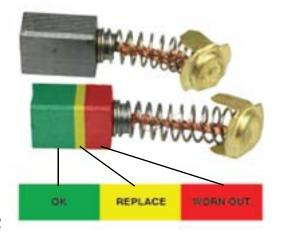
The motor on this machine has brushes. The brushes should be checked regularly to detect any abnormal wear.
