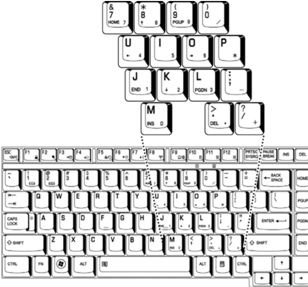
Figure 5-1 The numeric keypad overlay
