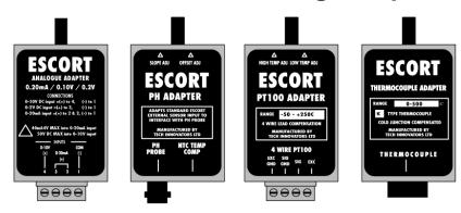
An Analogue Adapter is a device that plugs into any external sensor socket not dedicated to an external humidity sensor or pulse counting interface. An Analogue Adapter provides the functionality to let the logger connect to any type of sensor employing industry standard 0/4 to 20 mA or 0 to 10 Volt outputs. Specific adapters for PT100, Thermocouple and pH sensors are also available.
