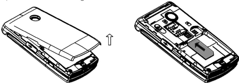
Insert the SIM card with the gold chip facing down and the slanted edge on the bottom right as shown. Carefully slide it under the silver bar.
