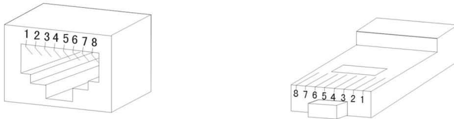
Fig. 4 RJ-45 Connectors, switch and cable views
