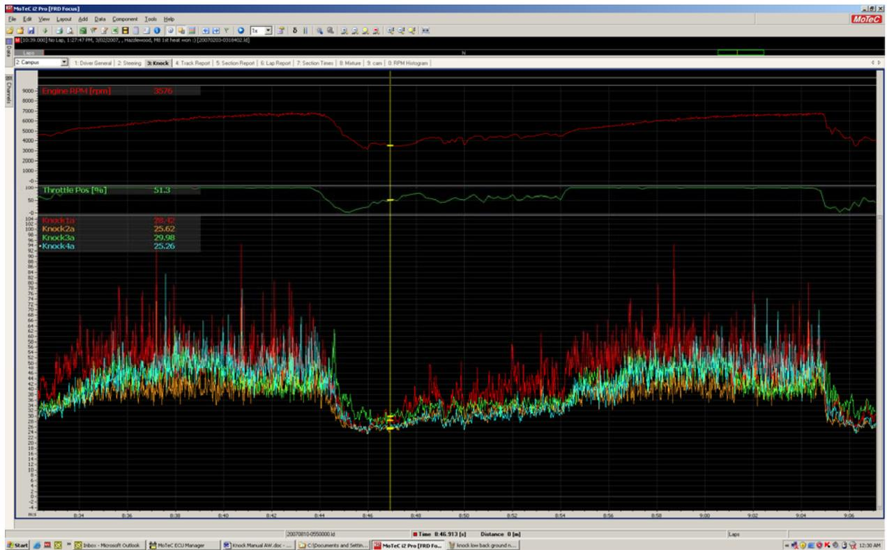
Log file from ECU with a centre frequency setting of 13 kHz
