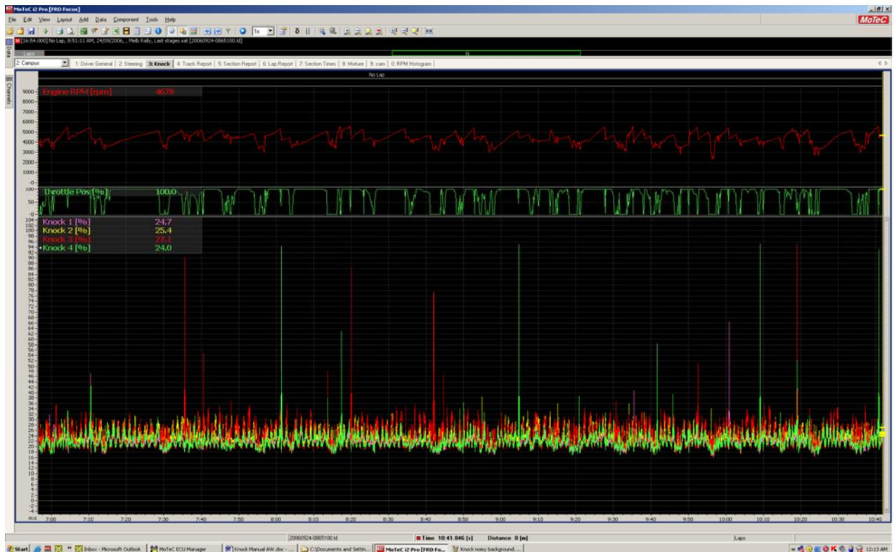
Log file from ECU with a centre frequency setting of 7 kHz
