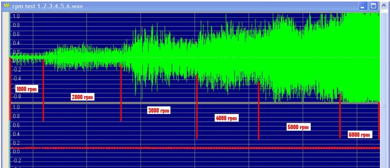
*Knock sensor signal with increased engine RPM*
