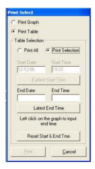
Click on the graph on the main screen to select your end time or click the latest end time button to automatically insert the latest end time.
