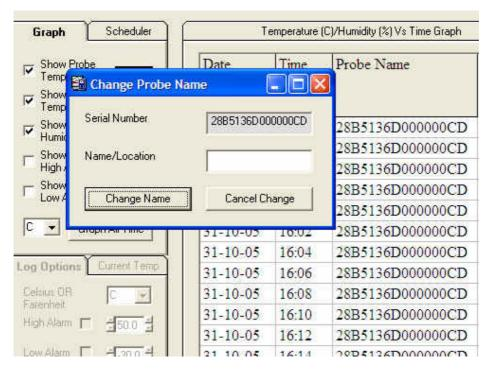
In the Name/Location text box type the new name for the probe and click the change name button.
