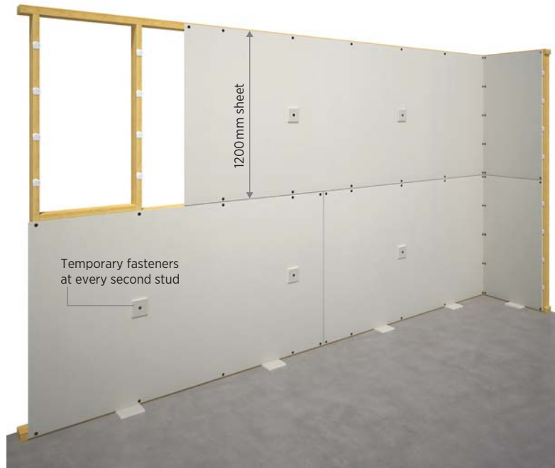
Figure 30: Combination adhesive and screw fixing on walls
