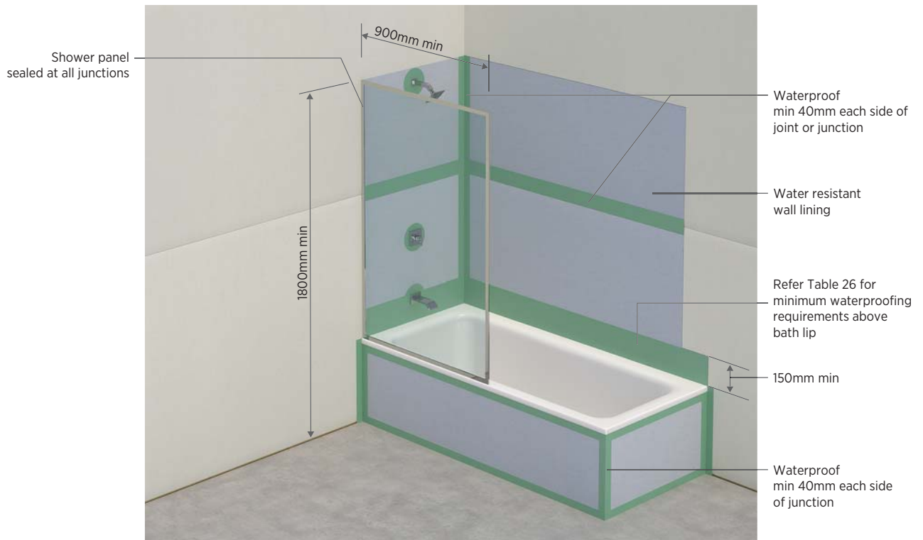
Figure 53: Waterproofing of enclosed shower over bath
