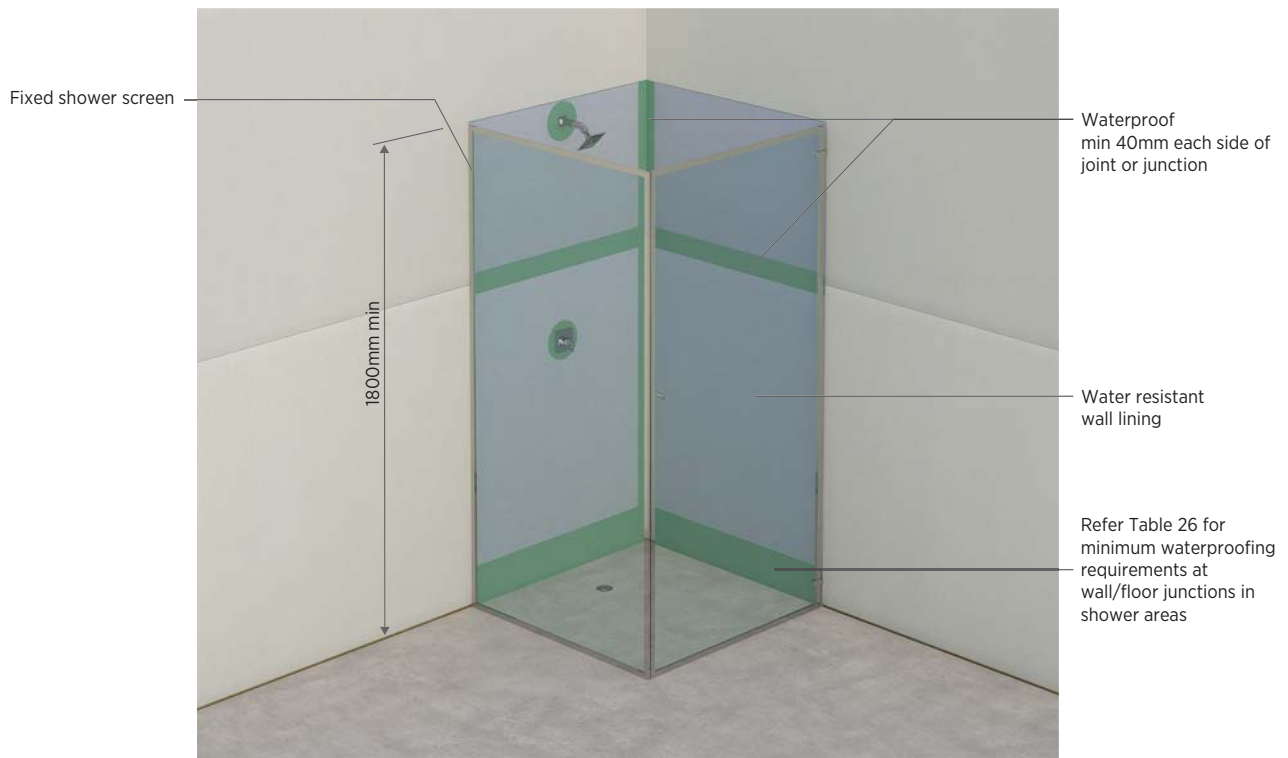
Figure 54: Waterproofing of enclosed shower
