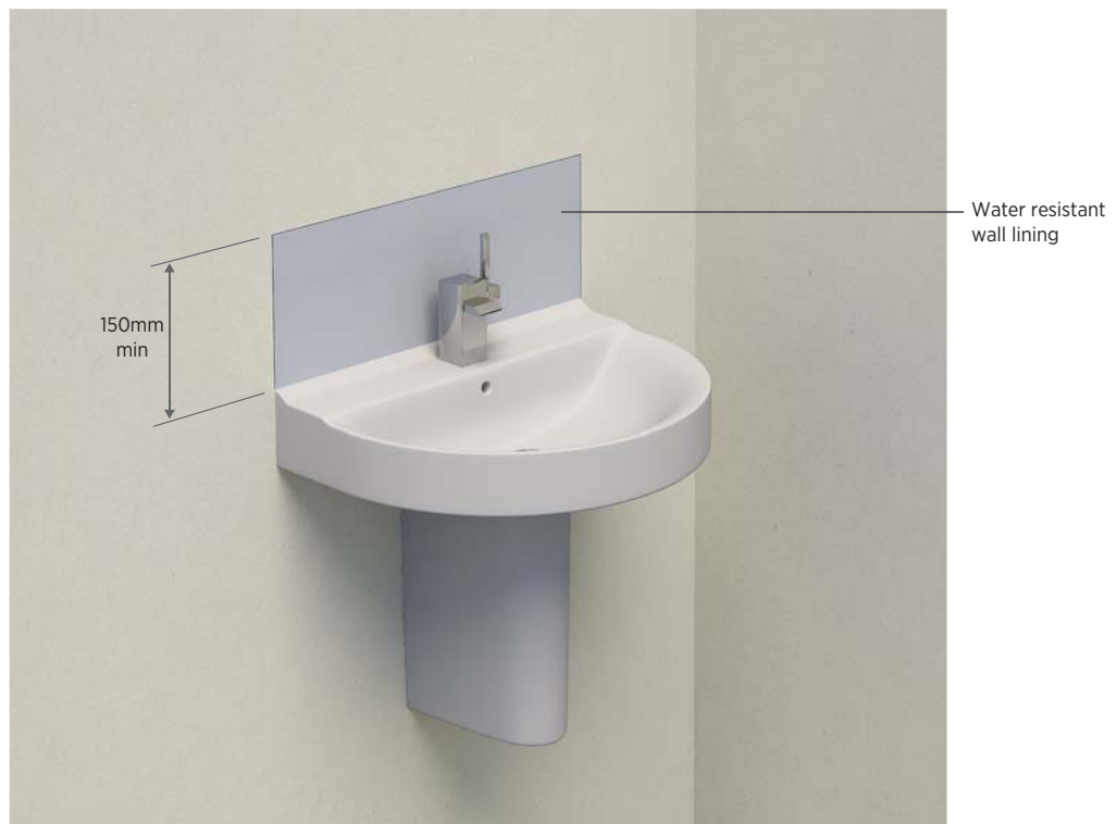
Figure 58: Waterproofing of basin
