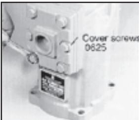
**To replace the valve plates and seal ring:** Remove the cover screws from the air eliminator cover with a 1/2 inch wrench or socket.
