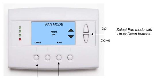
Press **DONE** button to select mode and exit back to main Thermostat Control Screen.
