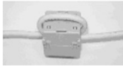
Figure 5-4: Ferrite used at PE inspection plate
