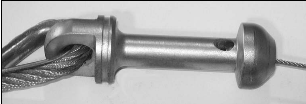
Figure 3-10: Pull-in Cable Fitted to Cable End
