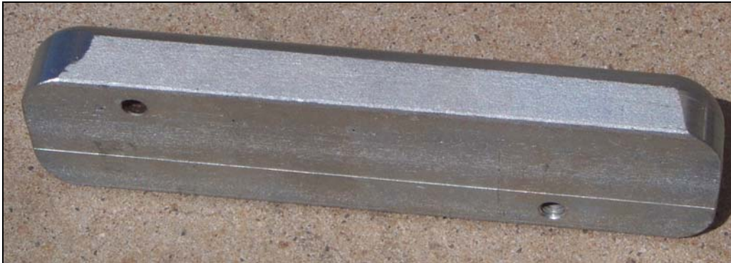
Figure 3-6: Extra Mass to be fitted to Counterweight Bar
