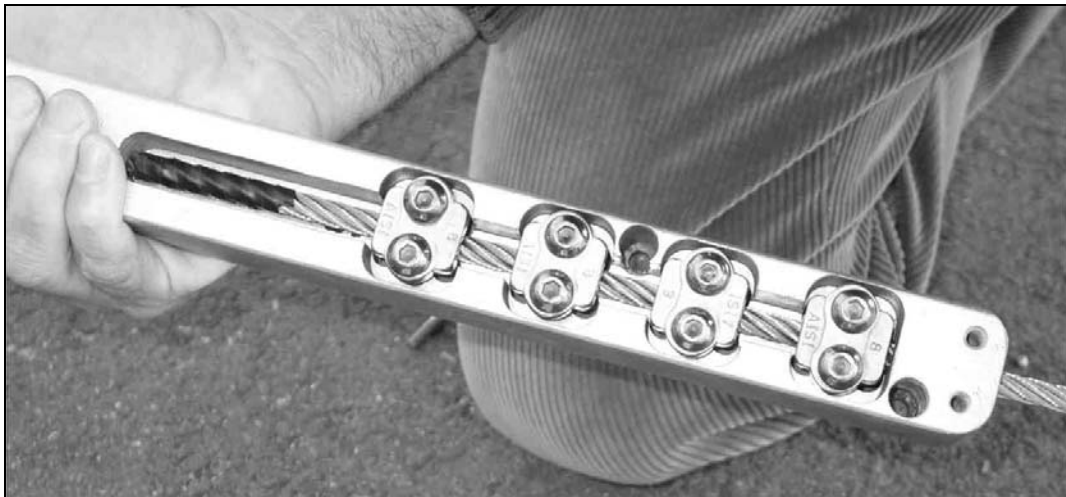
Figure 3-15: Inserting the Main Cable into the Counterweight Bar Slot
