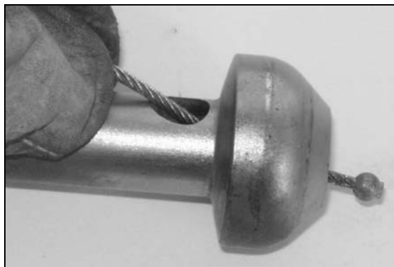
Figure 3-9: Pull-in Cable inserted into Cable End
