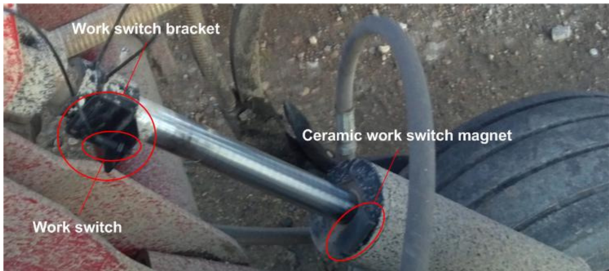
Figure 11: A work switch installed on an air seeder where no bracket previously existed In the figure above, the air seeder is out of the ground and the hydraulic cylinder is moved apart
