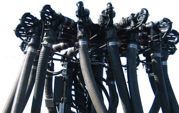
Figure 15: Flow sensors installed on a manifold
