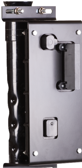
Figure 14: ECU installed on an air seeder tower
