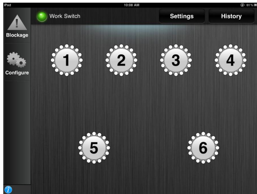
Figure 23: Renaming the ECUs example Top: Tractor connected to a six manifold air seeder, Bottom: Blockage screen representing that air seeder
