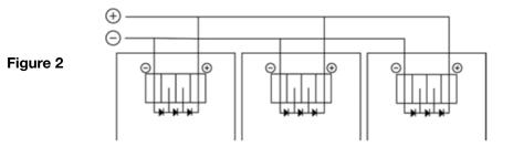
**NOTE:** It is recommended that paralleling modules be performed using an external junction box.
