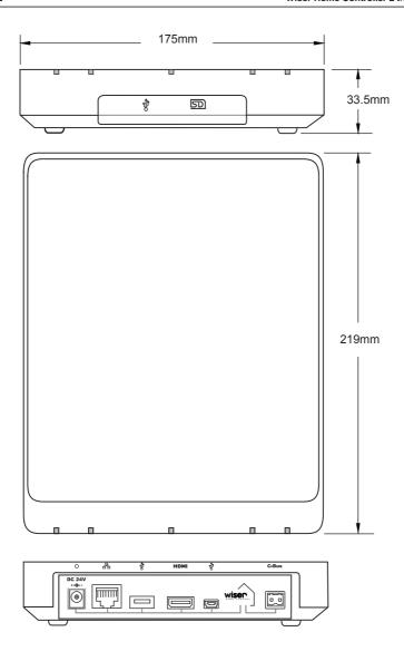
Allow 25mm (1 inch) space above and to the sides of the Wiser 2 to provide for adequate ventilation.
