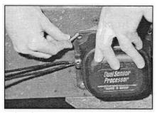
Use four of the 1/4 inch bolts and nuts and the 8 washers to mount the DSP to the frame. The washers should be placed on each side of the plastic DSP case at each hole.
