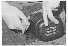
Hold the DSP in place using it as a template to mark the mount hole locations on the frame.
