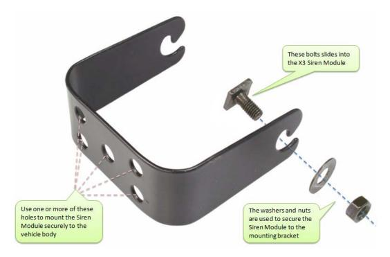
▶ Install the Siren Module to the mounting bracket using the screws and nuts provided. The siren can be mounted at a number of different angles to suit your vehicle as shown in the images below. Wherever possible, it is recommended to mount the siren with the opening facing downwards, towards the ground as shown in the examples below.
