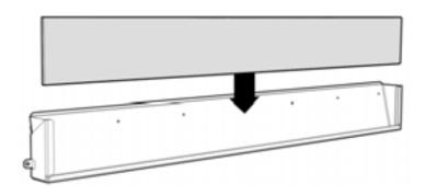
14.1 With the glass in position, fix the stone cartridge to the fire by using the two supplied screws in the location shown below. Do this before the fascia is fitted.
