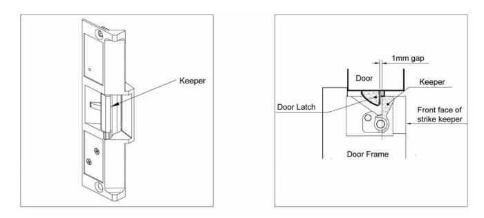
As drawn in the diagrams, there should be a 1mm gap between the door latch and the front face of the strike keeper, preventing the door from creating back pressure on the strike keeper when the door is closed.
