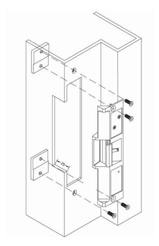
CUT-OUT DIMENSIONS AND MOUNTING TEMPLATE (not to scale)
