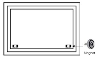
Put a screw into each of the magnets and attach them to the centre of each of the two backplates by using magnetic force (screw tips should face away from the screen).
