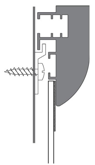
Lift the screen up against the wall, slightly higher than the brackets. Then let it slide down on the brackets until they are firmly in position. Only tilt the screen slightly during this operation, as it can loosen the brackets.
