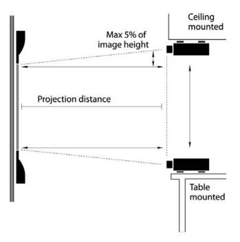
For the shortest optimal projection distance, see "minimum projection distance" in the Supernova One datasheet. It is possible to use a longer projection distance, but make sure that the projector can project the required image size onto the screen. In case of a mismatch, contact your projector reseller.
