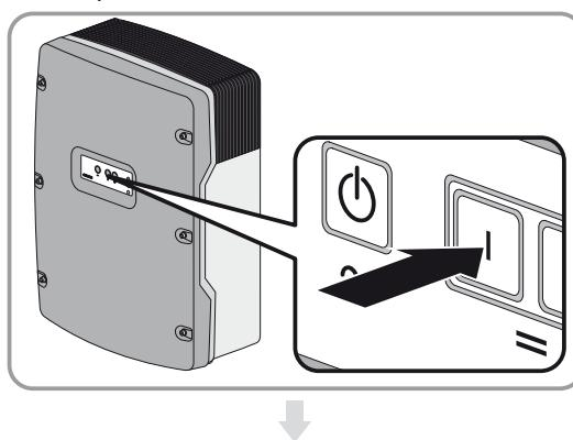
When the Sunny Remote Control shows **<Init System>**, press and hold the button on the Sunny Remote Control.
