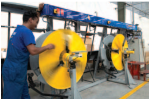
Manufacturing coils on the Buteline Pipewinder
