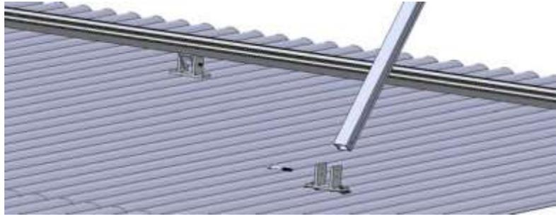
6. Adjust the length using a 4mm Allen key. Tighten M8\*10mm pressure bolt with 17Nm torque at the desirable height.
