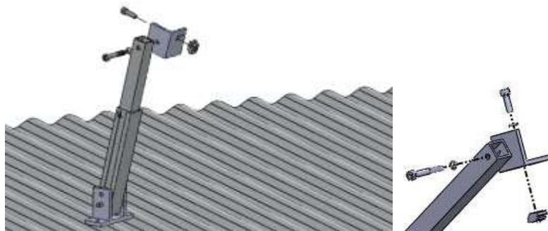
8. Insert the Z-Module on the L-shape bracket in to the channel on the side of the PV-ezRack<sup>®</sup> rail (recommended torque is 15-20Nm).
