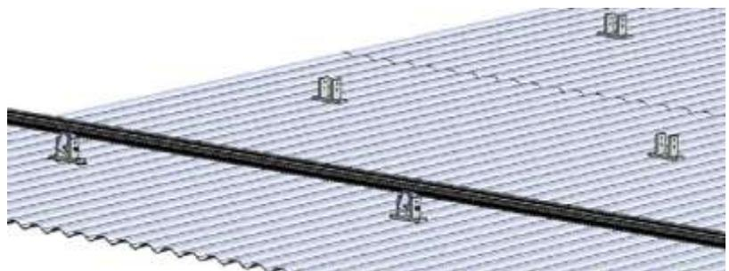
5. Install the back legs behind the front legs. Check the installation requirements (fixing points) of the PV-Module
