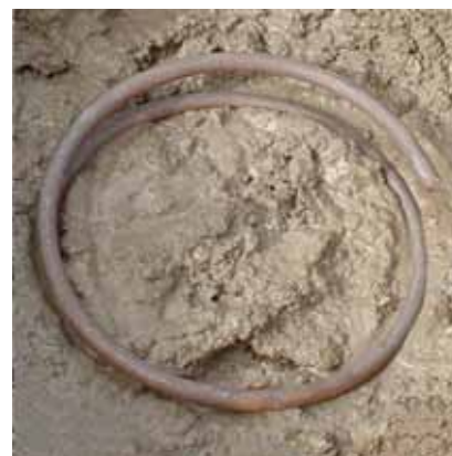
» Rebar ring (1 required per post)
