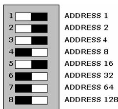
*Figure 14 - Temperature and Humidity Sensor Configured For Address 024*
