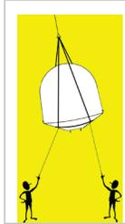
**CAUTION:** The antenna/radome assembly is very light for its size and is subject to large swaying motions if hoisted under windy conditions. Always ensure that tag lines, attached to the radome base frame, are attended while the antenna assembly is being hoisted to its assigned location aboard ship.
