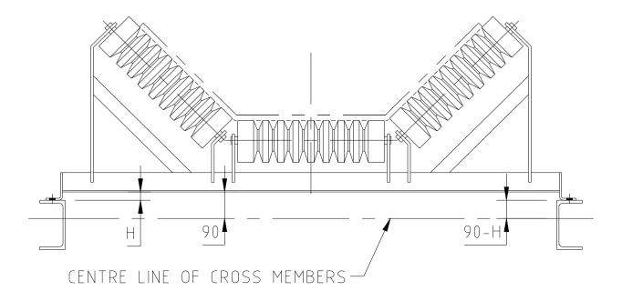
Determine the position of the Tracker Unit cross members. The cross members will be installed at exactly 500mm centres, and the guide frame of the unit will trail the front cross member by a further 750mm. Ensure the cross members are located to allow clearance from adjacent idler sets.
