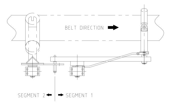
Take segment 2 from the previous step, comprising the rear cross member and the pivot plate. The Tracker is supplied with a matching plate bolted to the pivot plate. Remove this bolted plate and position it centrally on the bottom of the removed idler frame, studs down, making sure it is square to the centre line of the frame. Weld the plate to the frame.
