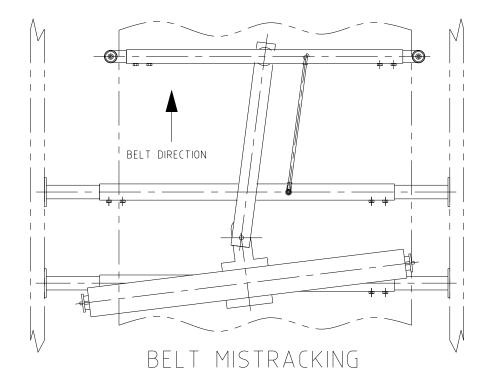
If adjustment is required, turn off and lock out/tag out the energy source to the conveyor and conveyor accessories. Check and tighten all fasteners after running the belt.
