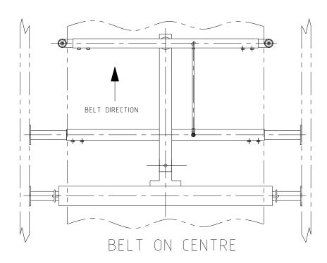
If the conveyor belt is mistracking, the ESS Tracker should be articulated around the front cross member pivot, and should be working to correct the tracking.
