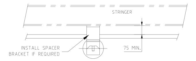
Remove the existing return idler at the installation position. Determine if the removed idler is to be used as the steering idler in the Tracker Unit. Any flat return idler in good condition can be used, but ESS recommends that a rubber lagged idler will have greater steering effect on the belt.
