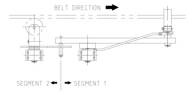
Take the front cross member and torque arm assembly (segment 1) and lift into place between the brackets, ensuring that the torque arm is downstream of the unit in terms of belt travel. Bolt this assembly into place on the pre-installed brackets, level and centre the torque arm.
