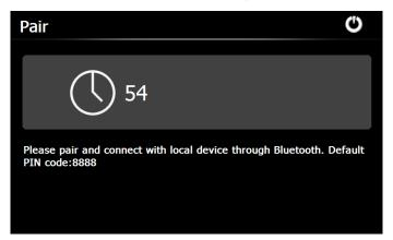
Meanwhile, press the icon "Search audio device" or similar one on the mobile phone. After the mobile phone finds and display the name of the navigator (i.e. PND), tap "Connect" and input the default PIN code: 8888. After pairing, the following interface will be displayed with connection situation and mobile phone name on the bottom.
