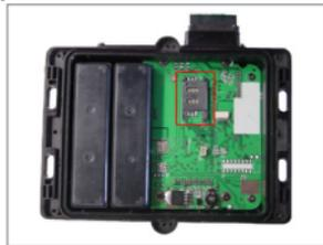
V) Insert the SIM card in the new device.
