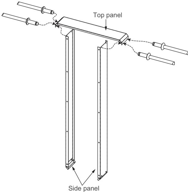
**Attach console panels to heater front cover**
