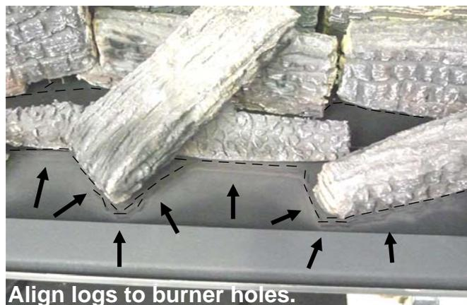
Align logs to burner holes.
