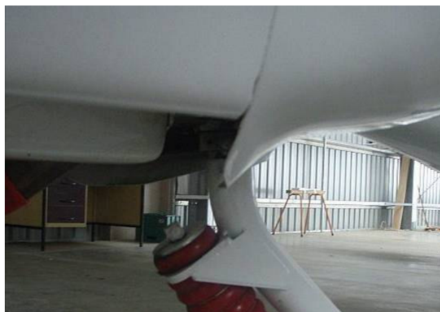
Figure 54: Lip to aid cooling as installed on a Jabiru.
