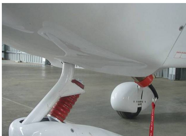
Figure 54: Lip to aid cooling as installed on a Jabiru.
