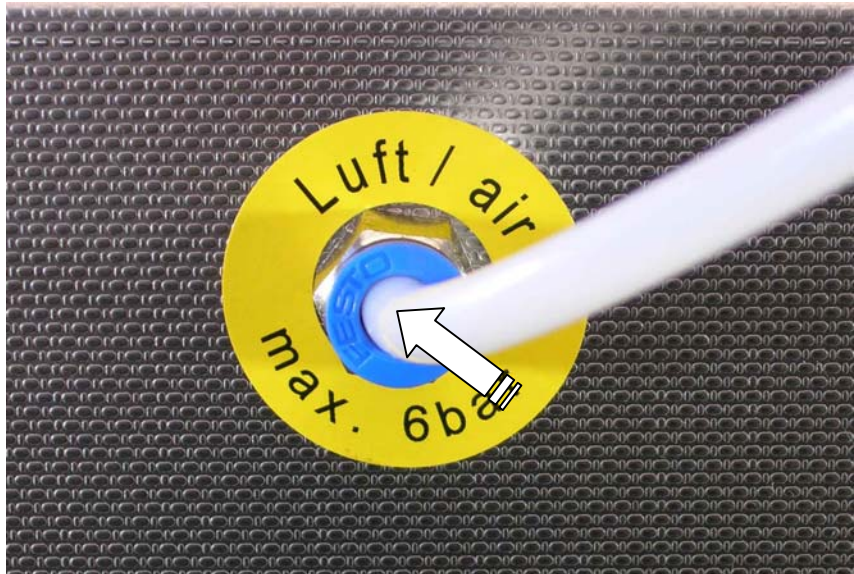
Illustration 6.1.1. Connect the compressed air duct at the correct connection socket
