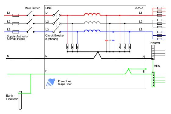
It is mandatory that Novaris filters be installed by a licensed electrician in accordance with Australian Standard AS3000 or the relevant country wiring rules. To meet AS3000 the filter must be protected by a circuit breaker or fuses of rating equal to the current rating of the filter. 63A filters may be fitted with line fuses. If these are not included the filter must be preceded by external fuses or a circuit breaker.
