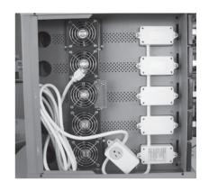
If no pedestal is being used under the stack, plug the top FUYL Cell into the 'hidden' socket inside the left cover of the FUYL Cell below then plug that FUYL Cell into the 'hidden' socket of the bottom FUYL Cell, then run the lead from the bottom FUYL Cell through the rubber grommet in the side of the bottom laptop space, through the back of the space and exit out the right hand side grommet where it can be plugged into an adjacent powerpoint.
