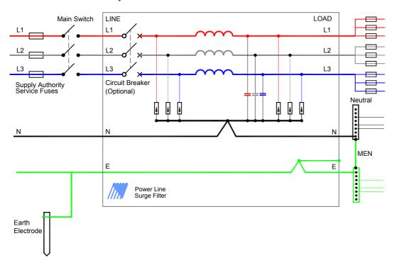
It is mandatory that Novaris Technologies filters be installed by a licensed electrician in accordance with Australian Standard AS3000 or the relevant country wiring rules. To meet AS3000 the filter must be protected by a circuit breaker or fuses of rating equal to the current rating of the filter. 125A filters may be fitted with line fuses. If these are not included the filter must be preceded by external fuses or a circuit breaker.
