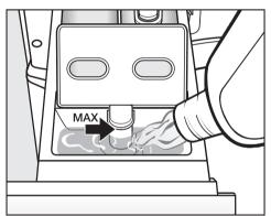
Add the fabric conditioner or liquid starch to compartment \mathscr{C}. Do not exceed the maximum level mark.
