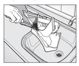
Clean the fabric conditioner channel using a brush and warm water. If starching frequently, thoroughly clean the siphon tube and fabric conditioner channel regularly. A build-up of starch will cause them to get clogged.
