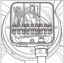
Figure 4: Connecting the wires to terminals
