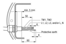
Figure 1: Recommended stripping lengths in mm (inside the terminal box)
