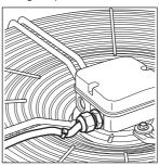
Figure 5: Fan installed lying flat (shaft vertical, rotor on bottom), cable routed as "water trap"
