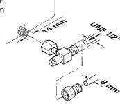
In industrial bulk packs the test connection is preinstalled and has to be tightened after the gas line has been connected. Please check for leaks before starting up for the first time. Check for gas leaks (do not check for gas leaks with a naked flame), then check that the gas pressure is as follows:
