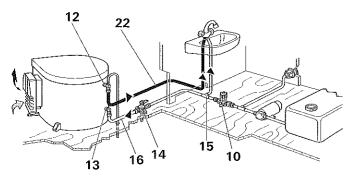
Produce connection (16) for cold water supply between Safety/drain valve (14) and elbow (13 - lower pipe) on water
