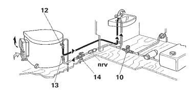
The supplied water connectors (12 + 13) and Safety/ drain valve (14) have a 12 mm rigid piping connection (e. g. John Guest System). For connecting to rigid pipes with other diameters appropriate adapters (not included in scope of delivery) must be used.
