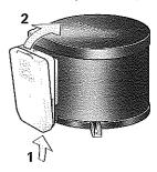
If the water heater is not to be used for a longer period, mount cowl cover (non-observance of this point can lead to the function of the appliance being impaired through water, dirt or insects), close stop cock valve in the gas supply line and close the gas cylinder.
