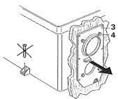
Screw the sealing frame (3) in contact together with the cowl body (1) so the anti-twist device projects out!
