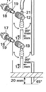
In industrial bulk packs the water connections are preinstalled and have to be tightened after the water pipes have been connected. Please check for leaks before starting up for the first time.
