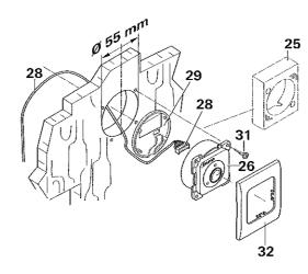
Drill a hole with diameter 55 mm.
