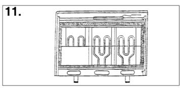
12. Fit the front layer of bricks again with the recess towards the element. The complete core will comprise:
