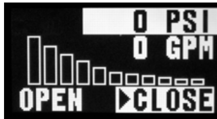
Figure #1 shows a Valve, Pressure Sensor and Flow Sensor connected.
