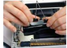
6. Attach the new battery to the connector.
