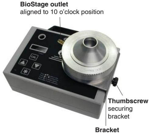
3. Insert the inlet adapter (included with bracket) into the pump inlet and connect inlet adapter tubing to the BioStage outlet.
