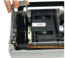
5. Carefully lift the battery pack out of the case and detach it from the connector.
