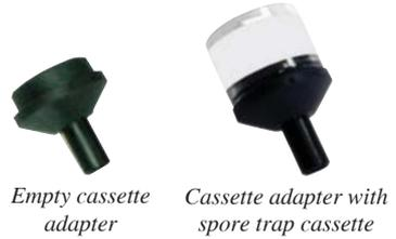
**Calibration Note:** Flow rate can be calibrated by pushing the bowl end of a second cassette adapter onto the spore trap cassette inlet (seal removed), attaching flexible tubing to the tube end of the second adapter, and attaching the other end of the flexible tubing to the outlet of a calibrator.
