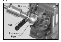
tion from damaging the threads. Once you have threaded the muffler into the exhaust pipe use an open end wrench and tighten the nut up against the exhaust pipe. This will prevent the muffler from loosening. The exhaust pipe is adjustable to better match the scale appearance and installation of your
