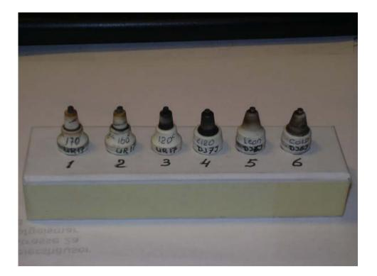
This plug looks about right. On disassembly, notice the black mixture ring in the isolator shoulder.
