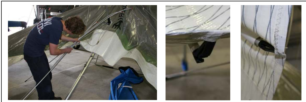
Figure 6 Section 4. Insert main sail battens
