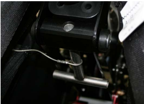
Figure 1 Mast over-centre loaded and secure
