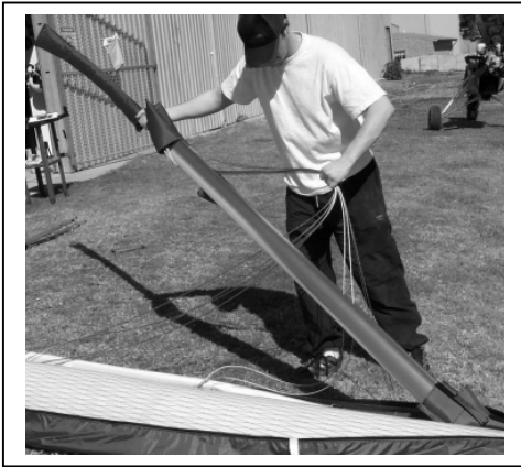
Figure 33 Section 4. Fit padding
