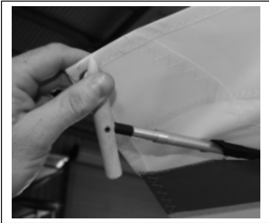
Figure 23 Section 4. De-tension tip strut
