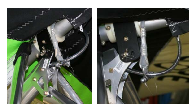
Figure 15 Section 4. Attaching the back up loop
