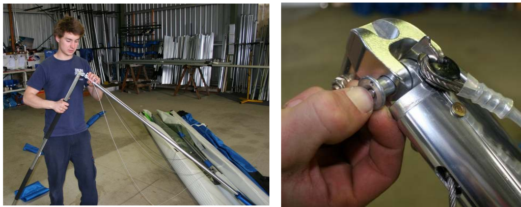
Figure 2 Section 4. Assemble control frame
