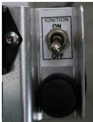
Figure 6 Section 2. Ignition placard locations.
