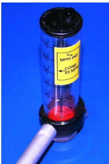
Figure 5 Section 7. T-Lite airspeed indicator.
