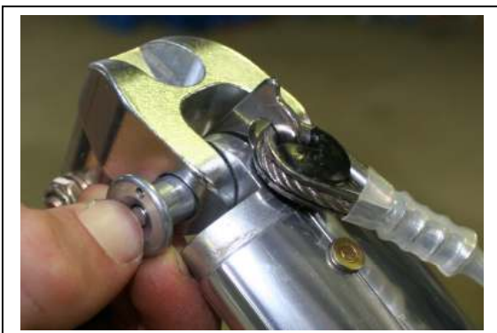
Figure 32 Section 4. Disconnect control bar
