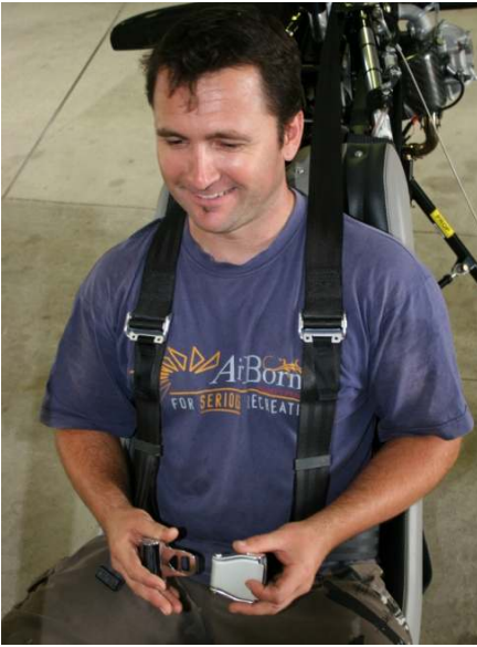
Figure 2 Section 7. Restraint harness, shoulder sash & buckle fitting.
