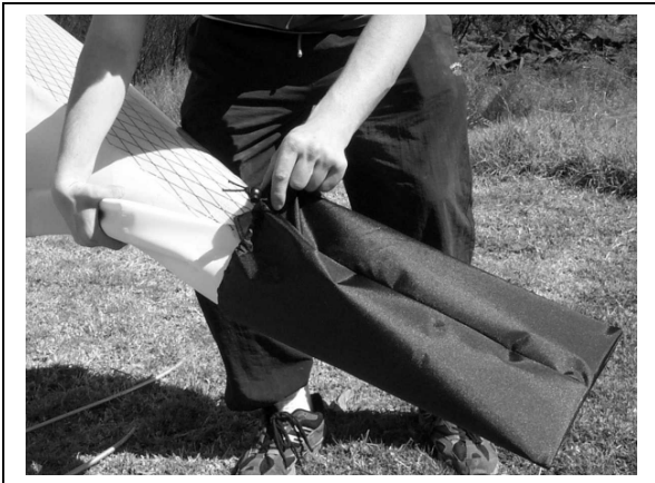
Figure 26 Section 4. Fit tip bags
