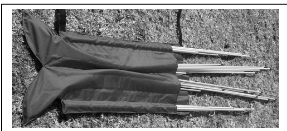
Figure 28 Section 4. Removing mainsail battens
