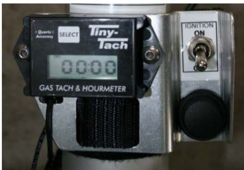
Figure 1 Section 7. Instrument Panel
