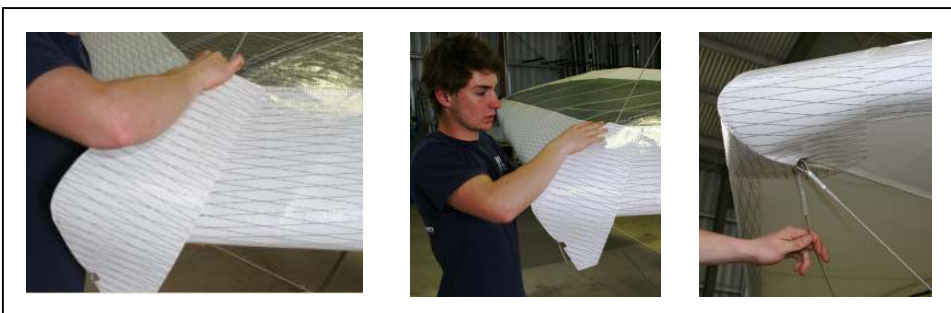
Figure 10 Section 4. Install nose nappy
