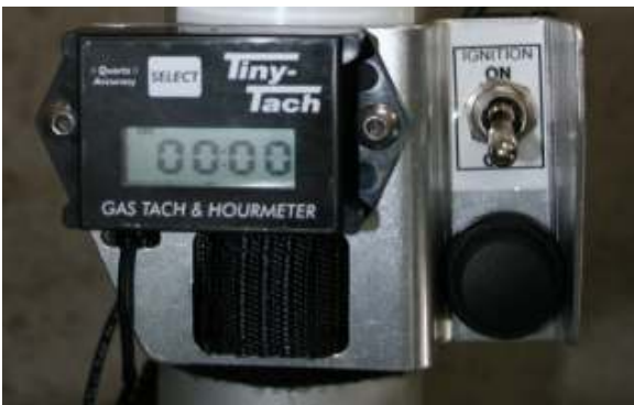
Figure 4 Section 7. T-Lite rpm / hour meter.
