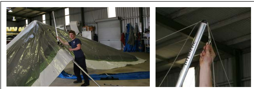
Figure 5 Section 4. Raise king post and connect reflex bridle
