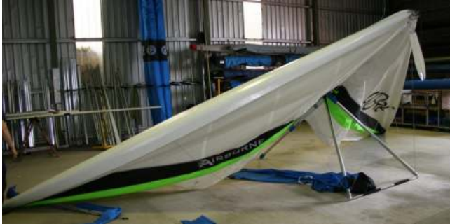
Figure 4 Section 4. Spreading the leading edges
