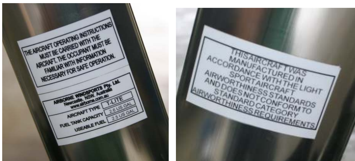
Figure 3 Section 2. Aircraft operating instructions, aircraft type & fuel capacity, and LSA placard locations.
