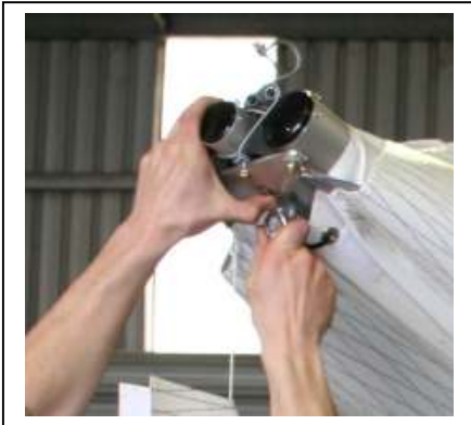
Figure 31 Section 4. Disconnecting nose wires
