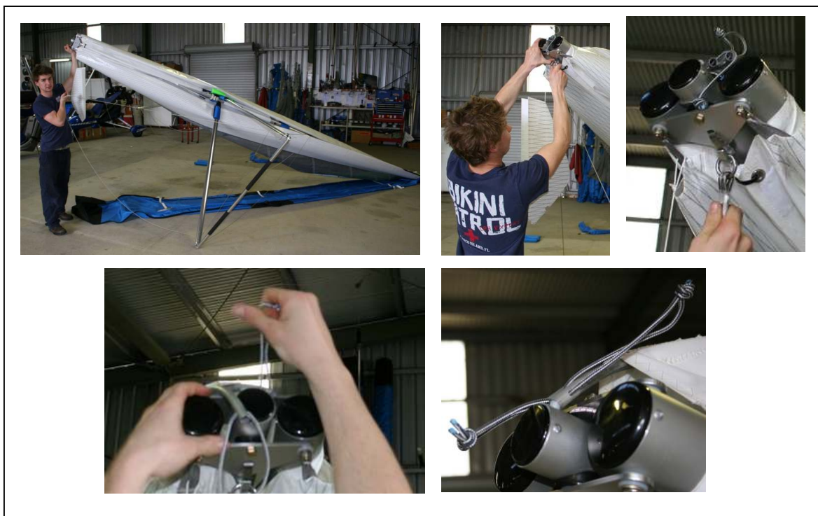
Figure 3 Section 4. Stand the wing up
