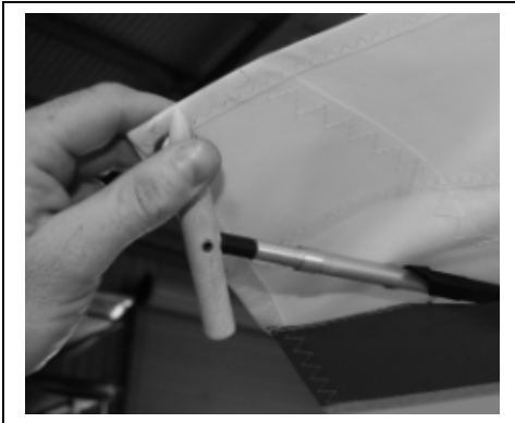
Figure 8 Section 4. Load tip strut
