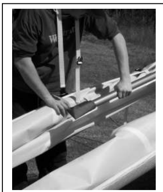
Figure 30 Section 4. Fold leading edges
