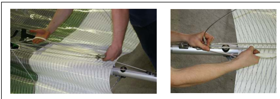
Figure 7 Section 4. Tensioning cross bar and shackle located in block
