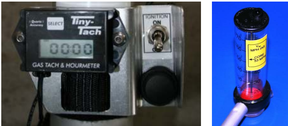
Figure 2 Section 9. Digital Instrument Panel (Tiny Tach & Hall airspeed indicator)
