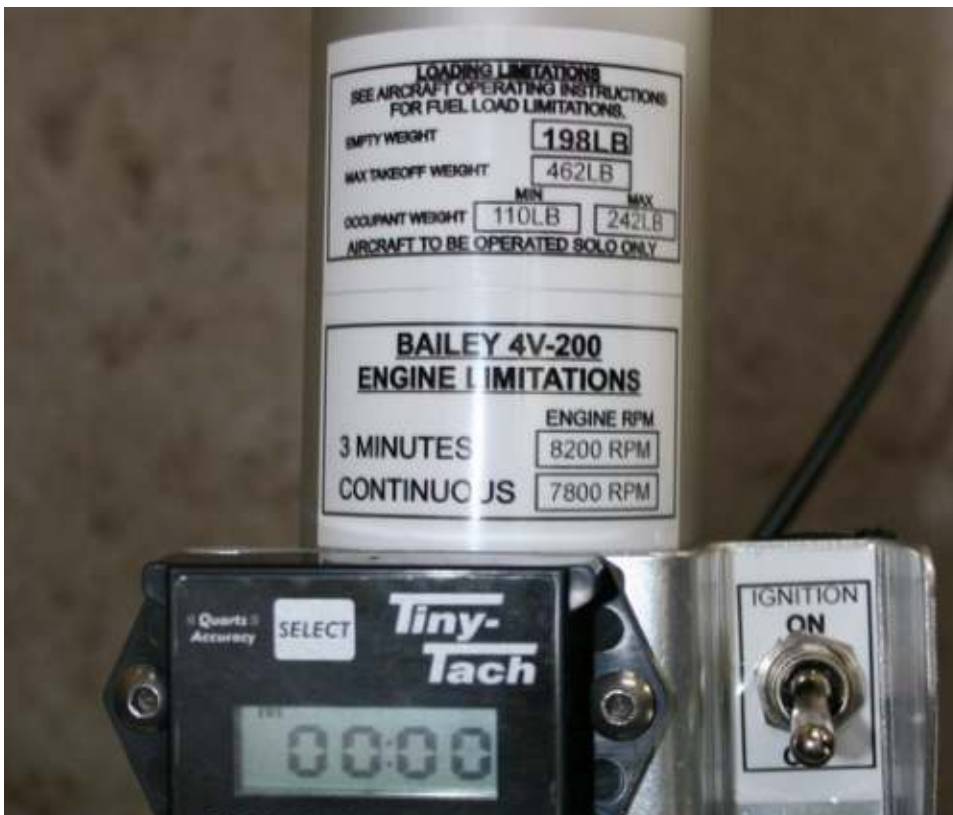
Figure 2 Section 2. Loading and engine limitations placard locations.
