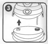
Line up the machine unit on top of the solution container.
