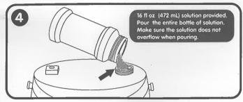
Slowly pour solution into the machine's solution container.
