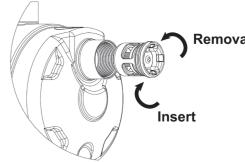
Removal of the check valve cassette is achieved by inserting any suitable tool (eg: a pair of pliers or the handle from an adjusting spanner) into the inlet. The check valve cassette has various ribs and recesses to allow a variety of nonspecific tools to be used in the removal or insertion process.
