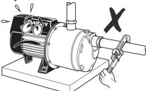
For best performance use P.V.C. or polythene pipe at least the same diameter as the pump's inlet. Larger diameter pipe may be used to minimise resistance to flow when pumping longer distances.
