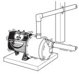
4. Prime should establish almost immediately with a strong flow of water, however, in some installations it may be necessary to repeat the above operation to remove all air from the system.
