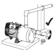
Use unions at pipe connections to enable easy removal and servicing. Use sufficient tape to ensure airtight seal and hand tighten only, do not screw connections all the way into suction port. To prevent strain on pump thread always support heavy inlet and outlet pipes. Lay suction pipe at a constant gradient to avoid
