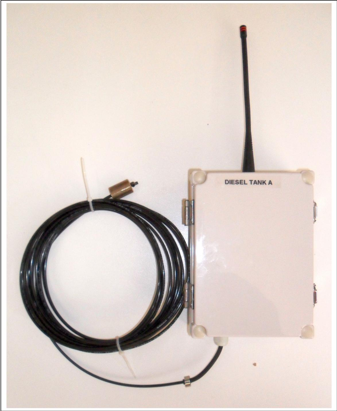
**Figure 1. Pressure sensor
